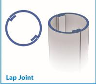
All fabricated in vertically split halves with a vertical lap joint, unless butt or reveal joints have been specified.
