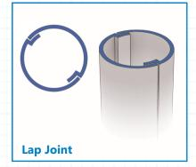
All fabricated in vertically split halves with a vertical lap joint, unless butt or reveal joints have been specified.
