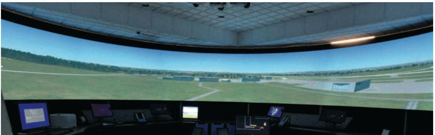
EDON, partnering with Display Solutions, designed, tooled and manufactured the Air Traffic Control Training Simulator at Middle Tennessee State University. The unique 360° fiberglass conical screen provides realistic images for advanced aviation training.
